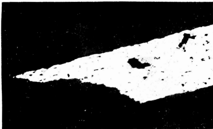
Fig. 13. Microphotographs ( \times 100 ) of one flake of alloy under some higher power, showing its two differential surfaces.
