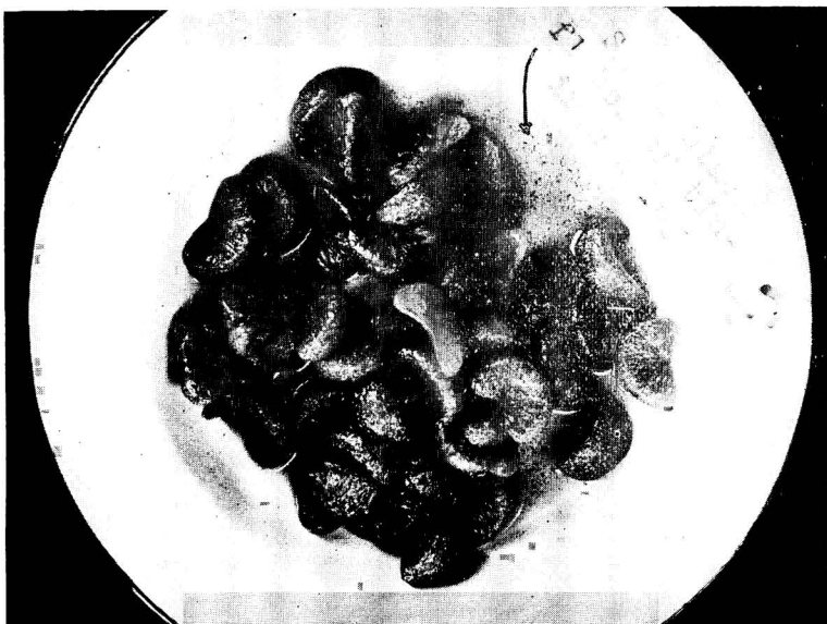
Fig. 10. Black small suspending matters (=flakes of thin film of tin-iron alloy) in a swelled canned oranges packed in the electro-tin plate can.
