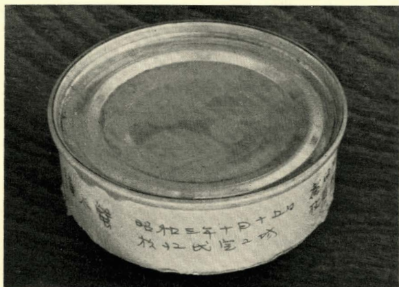
Fig. 1 External appearance of 35-year old aluminum can of crab meat.
