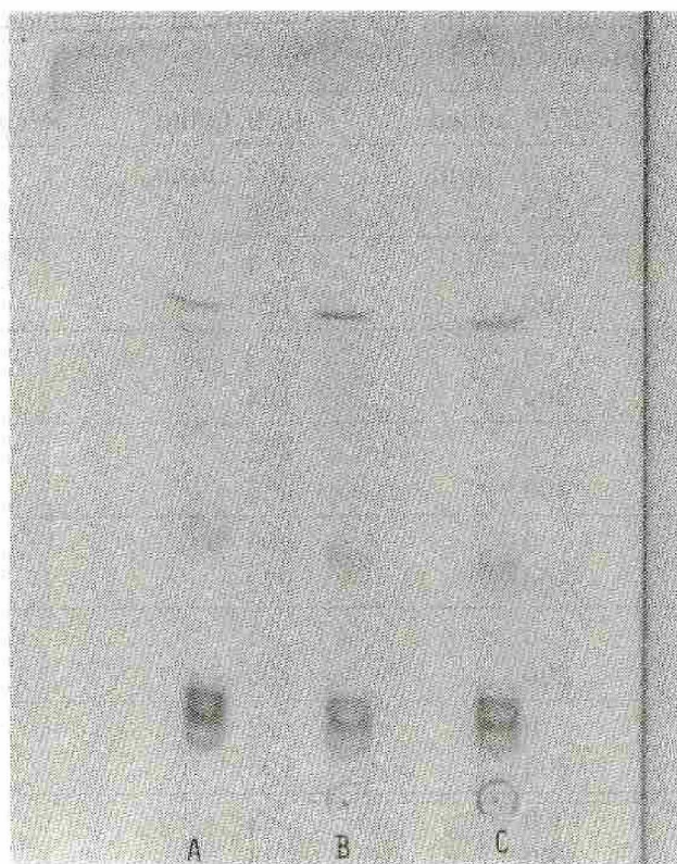
Fig.13. Thin-layer chromatograms of Sample No. 15 A: the emulsifier (P-1570), B: Sample No. 15, C: Sample No. 15 with 500 ppm of P-1570 added. Developing solvent: chloroform-methanol-acetic acid-water(80:10:8:2), chromogenic reagent: 50% H_2SO_4 2) .
