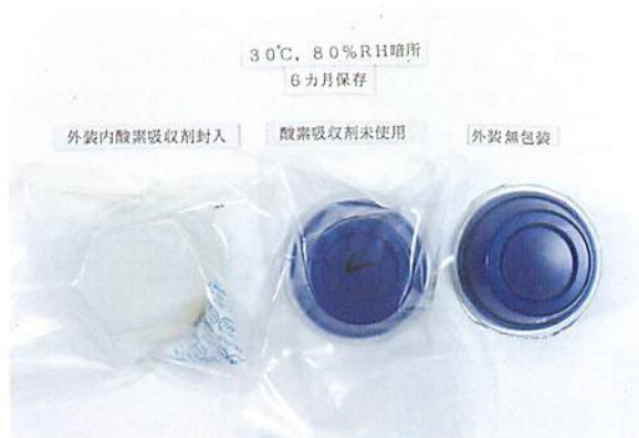
Fig. 4. Change of color for reoxidized methylene blue. Left: with an oxygen absorber Right: without an oxygen absorber
