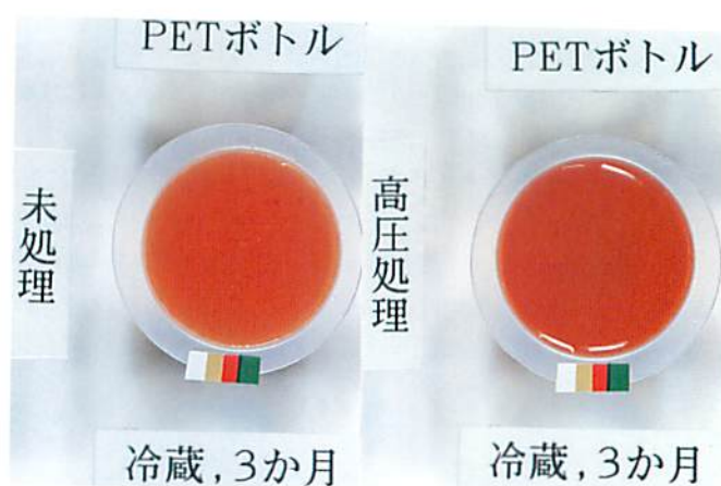
Fig. 6. Color of high pressure treated strawberry juice (3 month at 5°C) Left; Non-treated juice Right; High pressure treated juice
