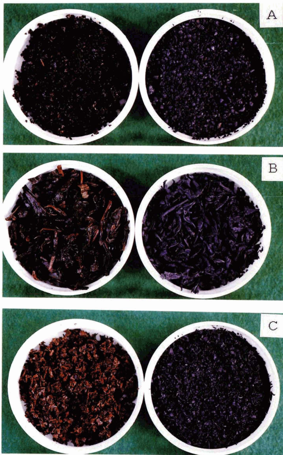
Fig. 3. Carbonized coffee grounds and tea wastes A. Coffee grounds B. Oolong tea waste C. Black tea waste Left; Raw material Right; Carbonized waste
