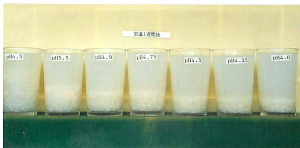
Fig. 5. Influence of pH on sedimentation of rice grains in canned "rice-gruel drinks".
